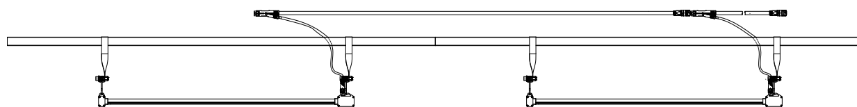
(E) Repeat step A,B,C,D,connect one daisy chain cable with other (1)for 820W grow light, the Max. links up to 8units (2) for 1640W grow light, the Max. Links up to 4 units
